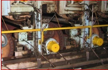
Fig 19: Gravity lubrication illustration
