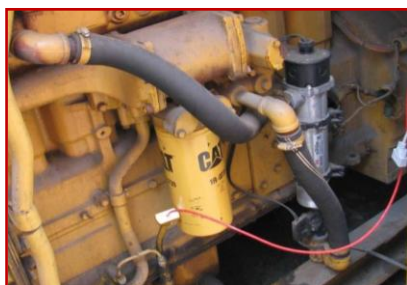
Fig 17: Dipstick Sensor detail
